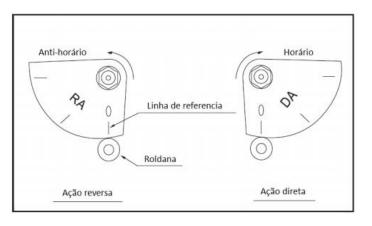
Zero Adjustment: Adjust the input signal to 4 mA, current required to keep the valve 100% closed. Then, move the "Zero Adjustment" in order to close the actuator and zero the pressure indicated on the manometer. Note that it is necessary to reduce the pressure to zero and not completely close the adjustment.
