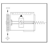
Span adjustment: supply the positioner with 20 mA, the necessary current to keep the valve at 100%. Adjust the span so that the actuator reaches the end of its stroke. After this step, return to zero (4 mA) and redo the zero adjustment. Note: every time it is necessary to readjust the span, the instrument must return to the zero position and the zero adjustment must be redone.
