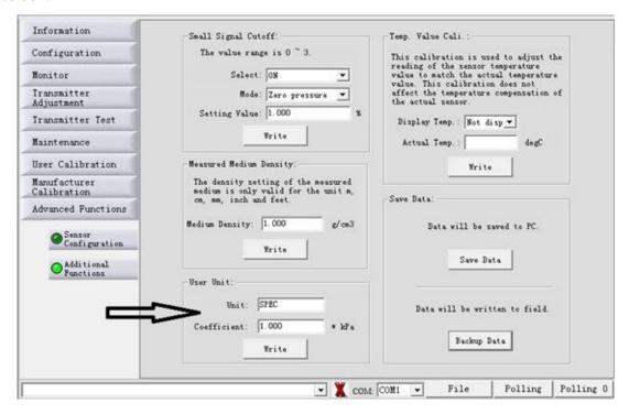
In the "User Unit" box, indicated by the arrow in the previous figure, write the user unit you want to use. Enter the value of the "Coefficient", which must always be the maximum value of the calibration range divided by the maximum value of the user unit range.
