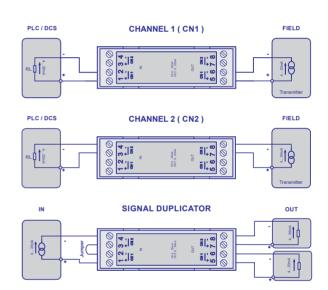
**IMPORTANT:** for the correct operation in duplicator mode, both outputs must be connected.
