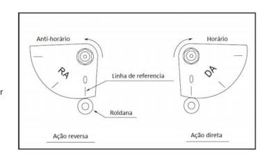
Zero Adjustment: Adjust the input signal to 4 mA, current required to keep the valve 100% closed. Then, move the "Zero Adjustment" in order to close the actuator and zero the pressure indicated on the manometer. Note that it is necessary to reduce the pressure to zero and not completely close the adjustment.
