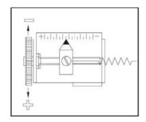
Span adjustment: supply the positioner with 20 mA, the necessary current to keep the valve at 100%. Adjust the span so that the actuator reaches the end of its stroke. After this step, return to zero (4 mA) and redo the zero adjustment. Note: every time it is necessary to readjust the span, the instrument must return to the zero position and the zero adjustment must be redone
